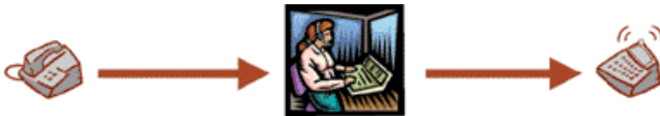
Figure 2.22. The voice telephone user rings a direct number to a relay service user with a text telephone. The relay service for text telephony is automatically invoked.
