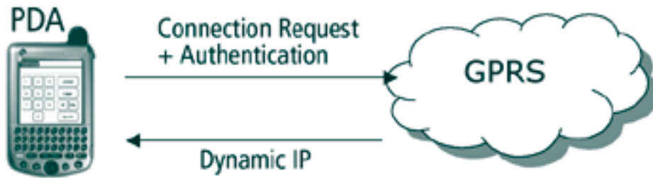
Figure 2.35 PDA connection with GPRS network. Dynamic IP assignment by the GPRS network. IP is fixed while connection is on.
